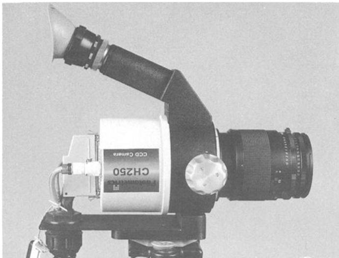
FIG. 4—Modified camera head with optical viewfinder.
